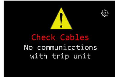
Figure 24: Check cables screen
