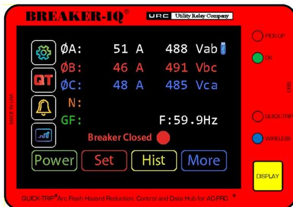
Figure 1: Front View with main screen
