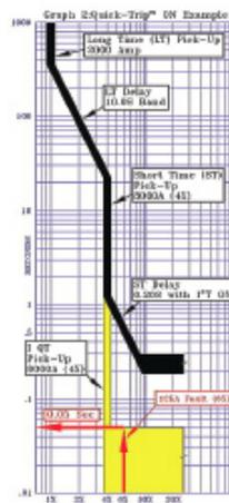
**Graph 2:** QUICK-TRIP® is ON & shows the trip time characteristics of the main breaker
