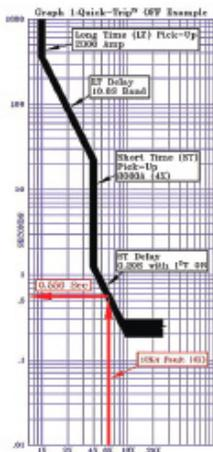
**Graph 1:** QUICK-TRIP® is OFF & shows the trip time characteristics of the main breaker
